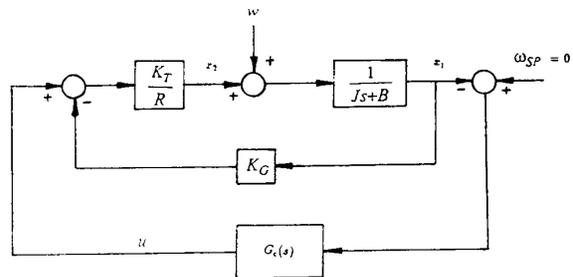
Figure 5: Block Diagram of the DC Motor-Speed Control System
