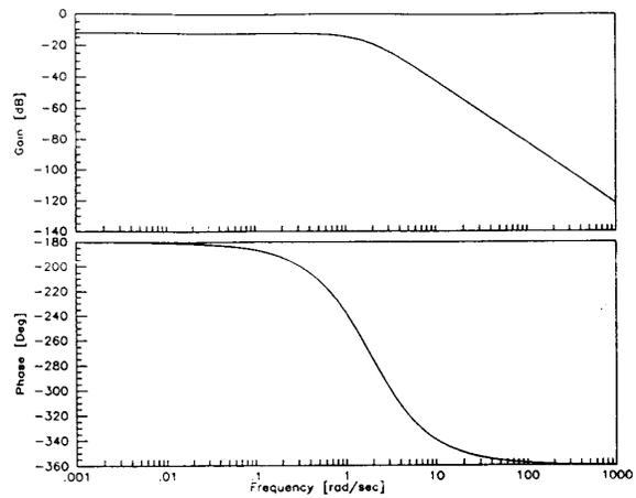
Figure 10: Frequency Response of  $L_o(s)$  - Design 2
