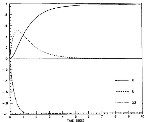
Figure 12: Time Responses for Step Disturbance ( $\alpha = 3.00$ ) - Design 2
