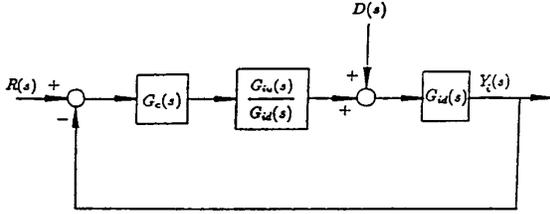
Figure 1: Block Diagram of the Feedback Control System
