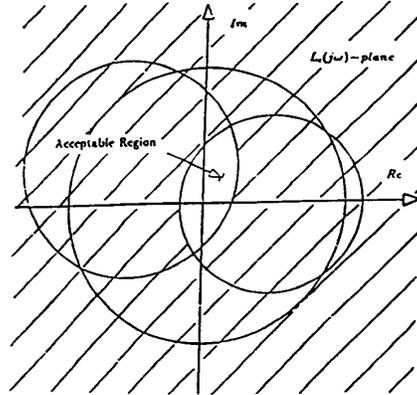
Figure 2: Allowed Region for a Closed Loop Transfer Function
