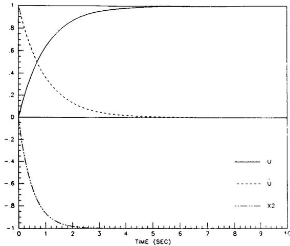
Figure 8: Time Responses for Step Disturbance ( $\alpha = 3.00$ ) - Design 1
