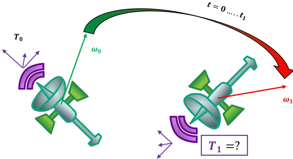
**Figure 2: Determine final attitude  $T_1$  from a rate change of  $\omega_0$  to  $\omega_1$**
