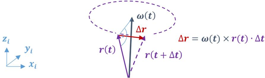
**Figure 3: Change of a vector due to rotation**
