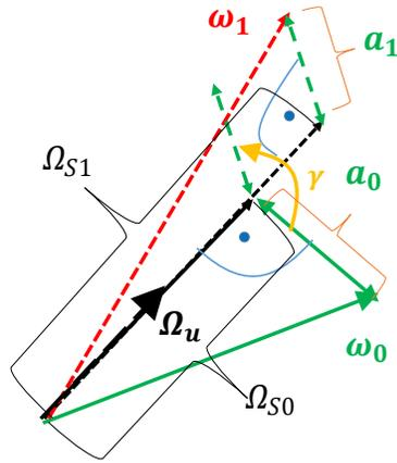
Figure 7: Preselecting initial rate  $\omega_0$ , final rate  $\omega_1$  and slew time  $t_1$  with corresponding scalar cylinder coordinates  $\gamma$ ,  $a_0$ ,  $a_1$ ,  $\Omega_{s0}$ ,  $\Omega_{s1}$
