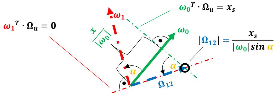
Figure 11: Construction of projection of rotation vector  $\Omega_u$ ,  $\Omega_{12}$ , into  $\omega_0$ - $\omega_1$ -plane
