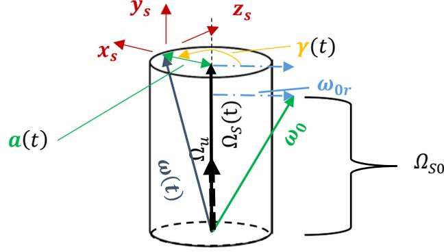
**Figure 5: Transformation from Cartesian coordinates into cylindrical coordinates**
